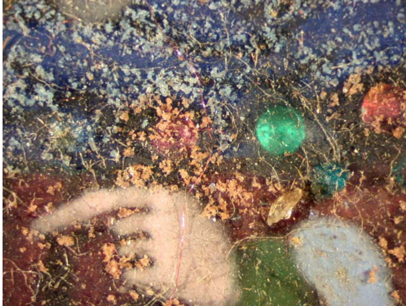
Detail of crizzled surface. Limoges painted enamel on copper, early 16 th c., Man of Sorrows , Walters Art Museum, 44.438. This unstable enamel crizzles below 48% RH and weeps above 52% RH. Photo: Terry Drayman-Weisser
