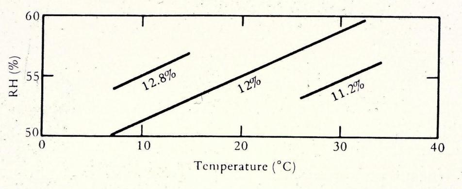
RH required to maintain constant EMC in wood under varying temp.
