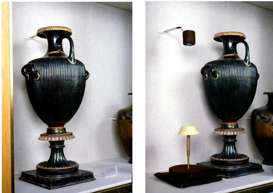
Figure 12: A static mount that secures the assembly of a multi-part vase to the deck the vase base) and the back wall of an exhibition case (the foot of the vase).
