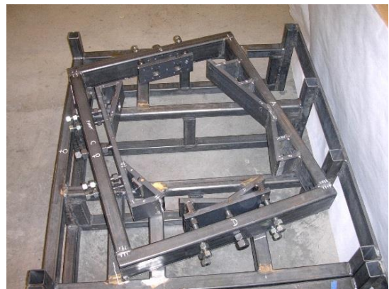
Figure 14: a schematic and a top view of the compression mount which was designed and built to secure two life size marble sculptures
