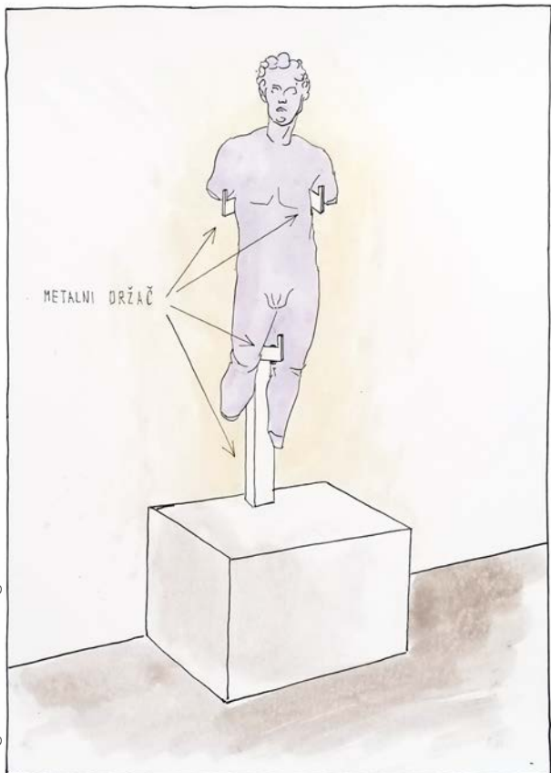
Metal support securing the object (drawing after the statue of Apollo kept in the Archaeological Museum, Zagreb) (Ivan Tudek)
