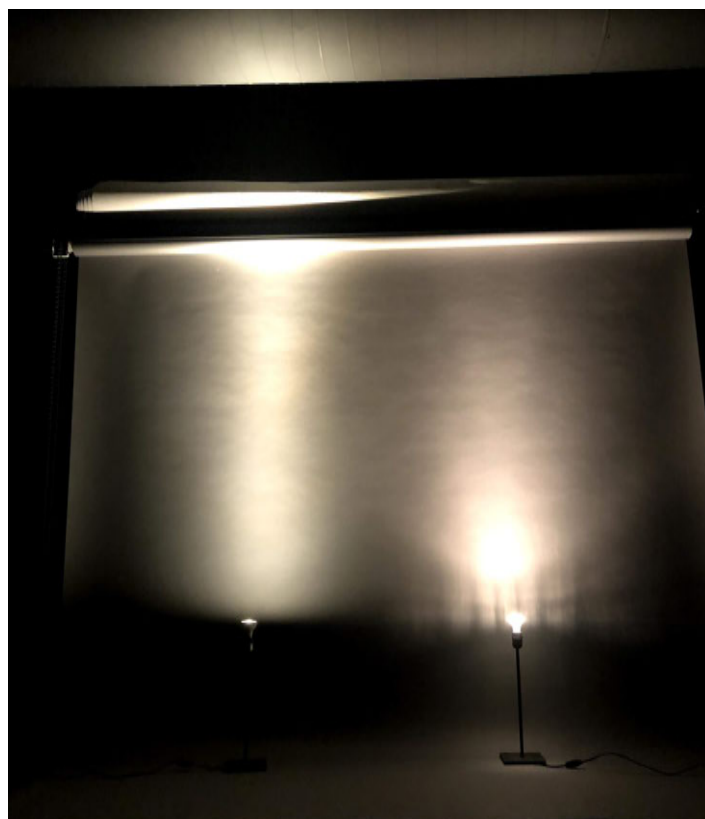
This image, taken during my time at MFAH, shows two potential replacement bulbs I ordered for the work I treated. Despite having similar manufacturer specifications, a side-by-side comparison revealed that many things about the light they produced were quite different! The resource I am preparing remotely will address this unexpected result. Image courtesy of Megan Salas
