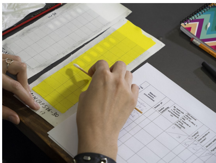
Participant testing different cleaning systems on acrylic paint, CAPS Argentina 2018. Photo Stephanie Auffret © 2018 J. Paul Getty Trust
