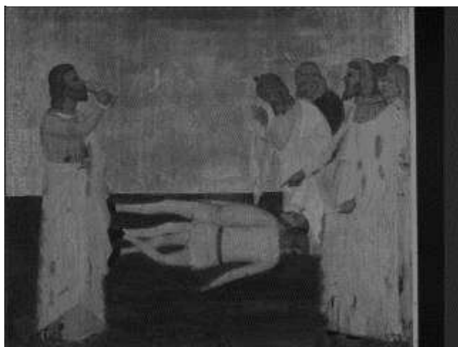
Fig.3 IR image (900-1700 nm) of NCMA St. John and the Poisoned Cup (60.17.20) (Goodrich SU640SDV-1.7RT/RS170 InGaAs Area Camera 640 x 512 pixel; 25 micron pixel pitch). Areas of retouching are clearly visible.
